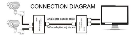
Warning: Need to use a single core coax cable to ensure the transmission distance.
