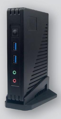
The Genie WMP300 is a management server specifically designed and developed for security surveillance application. Its software is installed before delivery and combines management, video preview and intelligent applications. Due to its simple deployment, flexible expansion, powerful performance and high reliability, it can meet the requirements of medium and small-sized security systems.
