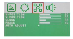
Set horizontal image position. H-POSITION: V-POSITION: Set vertical image position.
