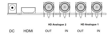
**DC:** Only use the 12v DC power supply included with the monitor.
