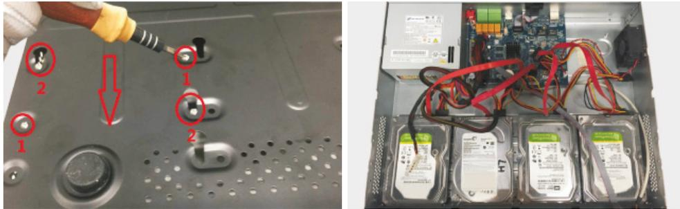
6. Install back the cover and secure it with the screws.
