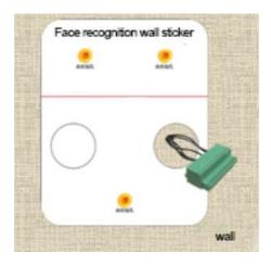
5. Move the bracket so that the three holes on the bracket align with the holes on the wall, and then secure the bracket to the wall with the self-tapping screws in the accessory.
