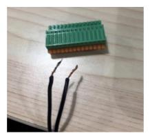
b) Press the orange button at each connector on the green bar to insert the wire end into the hole, then loosen the orange button to secure the wire as shown.
