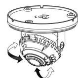
Please tighten up 3pcs of fixed screws with th L-wrench after closing dome cover.
