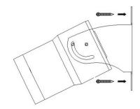
Adjust the angle of view with the 3-axis bracket.
