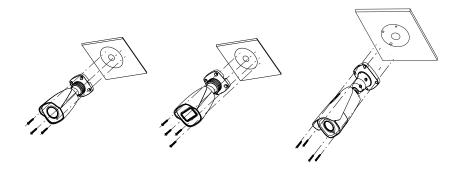
4. Bracket adjustment. Before adjustment, preview the image of the camera on a monitor and then loosen the fixed ring or screws to adjust the view angle of the camera.
