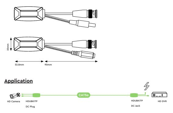
Use high quality CAT5e UTP or CAT6 UTP cable. The max working distance is 300m for AHD, CVI camera, HD-TVI maximum distance is 250m. The distance may affected by the quality of cable, camera, DVR.
